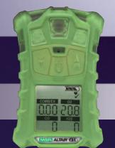
New optional glow-in-the dark housing for mining and confined space applications
