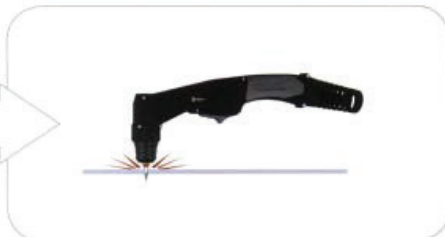
If sparks are spraying up from the work piece, you are moving the torch too fast, or you don't have enough amps set.
