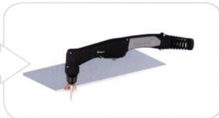
Pull the trigger to start the pilot arc. The cutting arc will initiate when the torch tip is close enough to the work piece. Start cutting on the edge until the arc has cut completely through.
