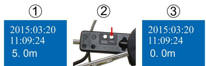
3. Hold the "METRIC/IMPERAL" button for 3 seconds, the meter count number hide; hold the button again for 3 seconds, the meter count number show.
