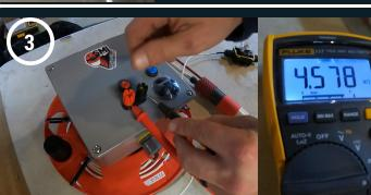
(3) Hook up the ohmmeter and take a reading. Loosen the collar device with the allen wrench and carefully pull the collar out of the hole enough to reduce the reading by approximately 400 ohms.
